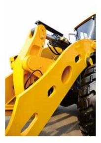
The double-row tapered roller bearings are adopted for the upper and lower hinge pins of front and rear frames, featuring high carrying capacity and high stability and reliability.
